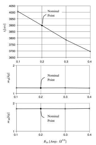
Fig. 19 Loiter time and mass breakdown as functions of no-load current parameter  $B_{Io}$ ; maximum endurance with ROC = 2 m/s.
