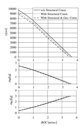
$\begin{tabular}{ll} Fig.~12 & Influence~of~additional~constraints~on~a~dual-goal~design~with~total~mass~constraint; Pareto~front~and~mass~breakdown. \end{tabular}$
