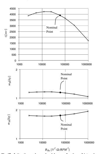
Fig. 17 Loiter time and mass breakdown as functions of internal-resistance parameter  $B_{Ra}$ ; maximum endurance with ROC = 2 m/s.
