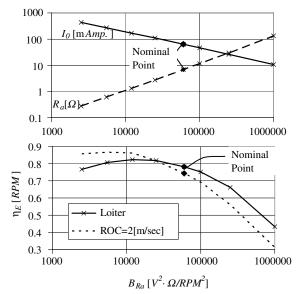
Fig. 18 No-load current, internal resistance, and electric system efficiency at loiter and ROC = 2 m/s as functions of internal-resistance parameter  $B_{Ra}$ .
