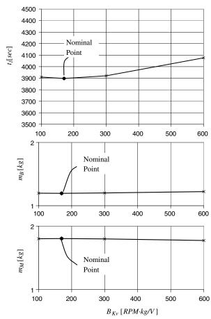
Fig. 15 Loiter time and mass breakdown as functions of motor speed-constant parameter  $B_{Ky}$ ; maximum endurance with ROC = 2 m/s.
