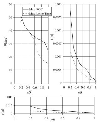
Fig. 6 Single-goal design: geometry of maximum loiter time and maximum-rate-of-climb propellers.
