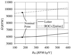
Fig. 16 Propeller rotational speeds at loiter and ROC = 2 m/s as functions of motor speed-constant parameter  $B_{Kv}$ .
