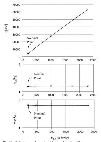
Fig. 21 Loiter time and mass breakdown as functions of battery energy density  $B_{EB}$ ; maximum endurance with ROC = 2 m/s.
