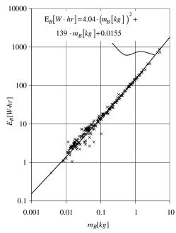
Fig. 5 Battery capacity as a function of battery mass.
