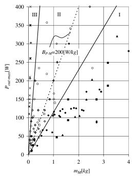
Fig. 1 Motor maximum output power as a function of motor mass.
